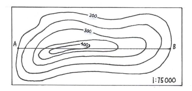
2) Construct a cross-section profile for A to B. Use a Vertical Scale of 1cm represents 200m. Also calculate the vertical exaggeration for the profile.
